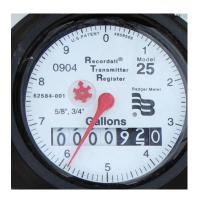
Typically, there will be a small triangle or star (shown) sometime in a different color than the dial (red or blue) that is a leak detector and will continue to spin clockwise when everything is turned off, but you still have water flowing because of a leak.
